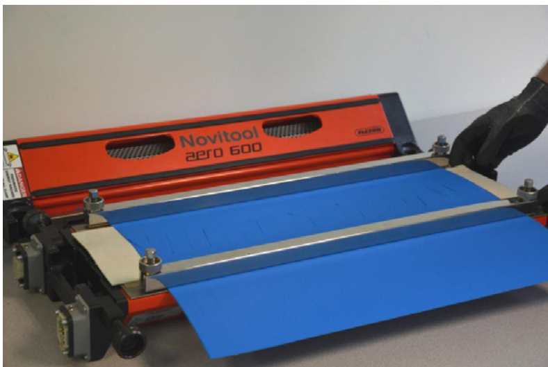
Filler Strips Added
