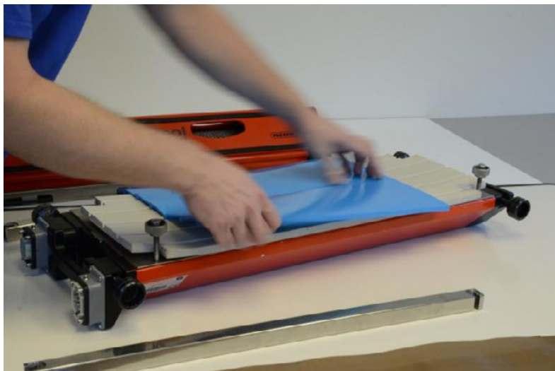
Belt Loaded in Opposite Side
