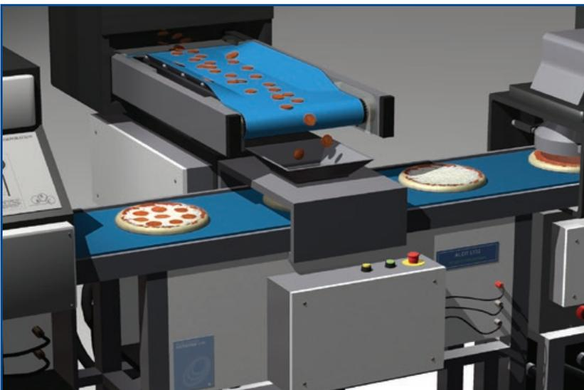
*CenterClean belts are constructed with flexible urethane and sealed Kevlar® tension members. This construction allows CenterClean belts to be troughed or run on small diameter pulleys with minimal belt stretch.*
